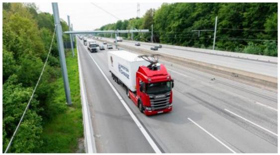
Figure 11 – Electrified road system trial<sup>52</sup>
